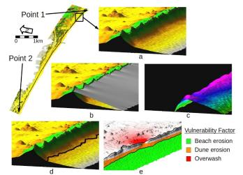
Figure 1. Coastal feature extraction using the LCP method: (a) DEM with extracted dune ridge, (b) DEM with sheet anchored at dune ridge and shoreline, (c) surface showing the elevation difference  $\Delta z$  between the DEM and the sheet, (d) dune ridge and dune toe, (e) vulnerability factor draped over DEM.
