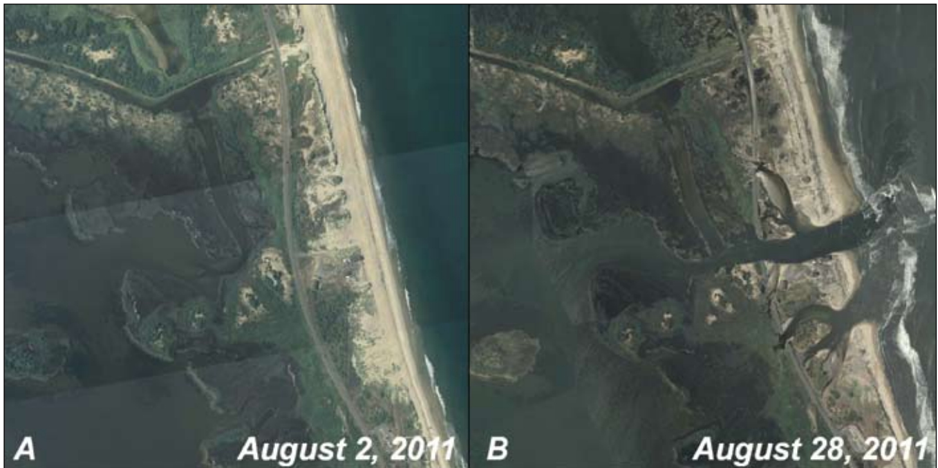
Figure 3. Pea Island breach site before and after Hurricane Irene. (A) was taken on 2 August 2011 before Hurricane Irene reached the Outer Banks on 27 August 2011. (B) was taken after Hurricane Irene on 28 August 2011 (NCDOT imagery).
